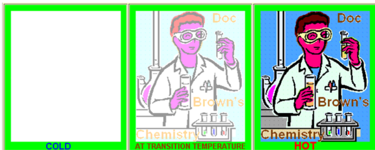
Figure 1: Application of thin layer thermochromic pigment paint in a preprinted coffee mug. At room temperature (COLD), the picture does not appear; but pouring a hot drink into it, at a specific transition point, such as 35 °C, the plain layer thermochromic pigment starts to turn transparent. The image in its entirety eventually appears (middle photo). The fully colored image appears heated (right picture). Retrieved from ref 4
